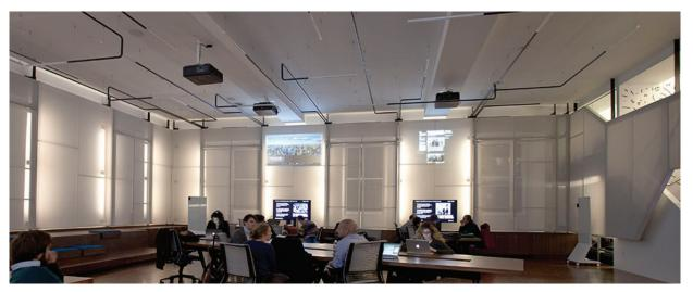
"We needed to address reflection of backlight fixtures on the scrim that came from the windows at night", commented designer Gabe Guilliams."The FLX Stix magnetic mount provided an easy means to adjust the placement of each fixture to avoid reflection. This was done simply and efficiently by our design team on-site without having to involve the contractors.
